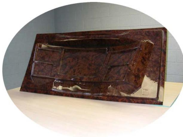
Fiberglass interior dash panel converted into a thermoformed dash. **Advantages:** *Cost- reduction, light -weight, aesthetic appeal, complex styled shape.*
